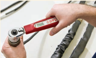
Digital torque wrench, adaptor, connector, strain relief
