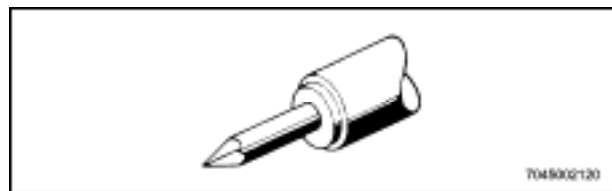
Figure 12-14 Correct Shape for Soldering Iron Tip
