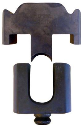
Rounding matrix 25R21ML and rounding punch 25R21DL.
