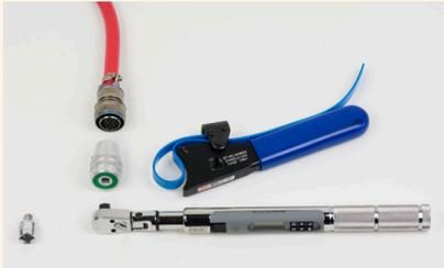
*Digital torque wrench, adaptor, connector, strap wrench*
