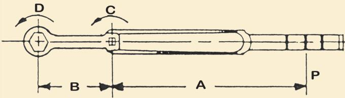
When an adapter or extension is used on a torque wrench it increases the torque range of the wrench. The formula for computing torque when using an adapter or extension is explained below.
