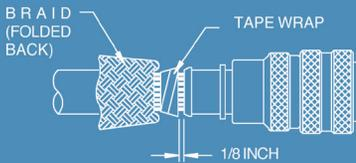
Use self-vulcanizing tape or a preformed component to build up the area behind the backshell. It is important that the braid is supported in the transition from the backshell rear diameter to the natural diameter of the wire bundle. Leave approximately 1/8 inch spacing between the tape wrap and the backshell.
