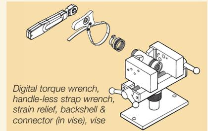
*Digital torque wrench, handle-less strap wrench, strain relief, backshell & connector (in vise), vise*
