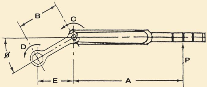
Should it be necessary, due to obstructions, to have an angle between the two axes, then the above formula is modified as follows. Due to increasing rounding errors, keep the angle as small as possible.
