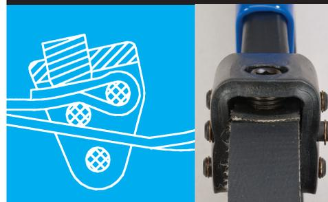
The strap is inserted into the buckle, folded back over itself, and clamped in place with a 7/32 inch set screw.
