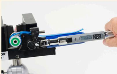
*Digital torque wrench, strap wrench, connector, vise*
