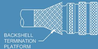
The braid is then carefully moved from under the backshell. It is important to retain the woven characteristics of the braid during this step.
