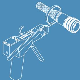
A shield termination band is then loaded into the tool. The band is then slid over the connector/backshell assembly into a position of alignment with the termination platform.
