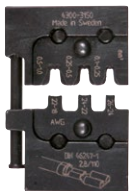
ORB0110 Crimping die for Elpress MOBILE tool for roll crimping uninsulated terminals 0.1-1 mm 2 . AWG 26-17.
