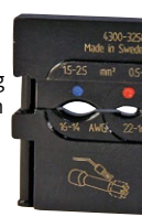
OSW0525 Crimping die for Elpress MOBILE tool for crimping through connectors with heat shrink insulation 0.5-1.5 mm 2 and 1.5-2.5 mm 2 . AWG 15-13.
