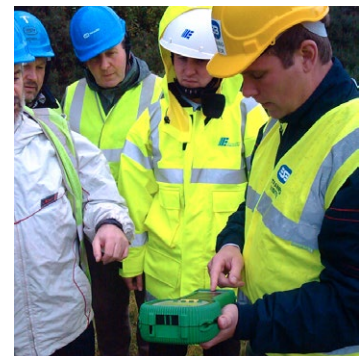
Measuring earthing resistance of the earth connection
