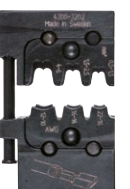
ORB0560 Crimping die for Elpress MOBILE tool for roll crimping uninsulated terminals 0.5-6 mm 2 . AWG 20-9.
