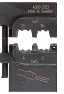
OEB1625 Crimping die for Elpress MOBILE tool for crimping end sleeves 16-25 mm 2 . AWG 5-3.
