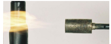
Shrinkage of the insulation is achieved by using heat.
