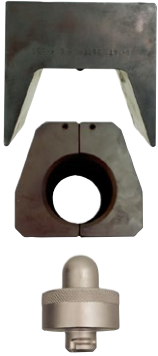
Matrix holder V1471, Matrix W60M, punch W60D.
