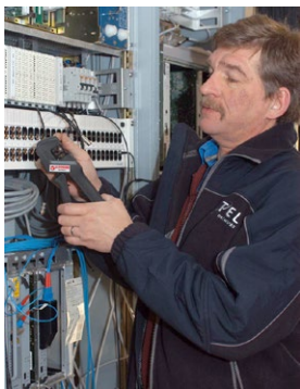
Elpress Mobile, professional tool with interchangeable dies for the installer or service technician.
