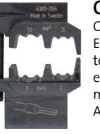
OEB1625 Crimping die for Elpress MOBILE tool for crimping end sleeves 16-25 mm 2 . AWG 5-3.
